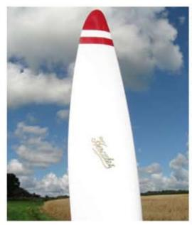
Hercules Propellers has made a number of "small but significant" improvements to its range of bespoke airscrews. The first innovation is a 'Spitfire Tip' - a slight reshaping reminiscent of the fighter's
