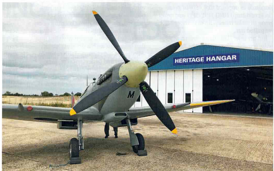
Test aircraft for Hercules's new propeller blades, Mk IX Spitfire TA805 The Spirit of Kent
