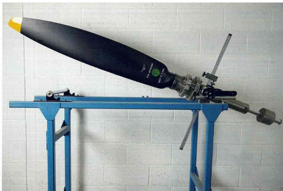
ABOVE: the static balancing rig is so sensitive, it can be disturbed by someone walking past - Hercules now produces propeller blades so precisely matched that sets from different batches can be mixed
