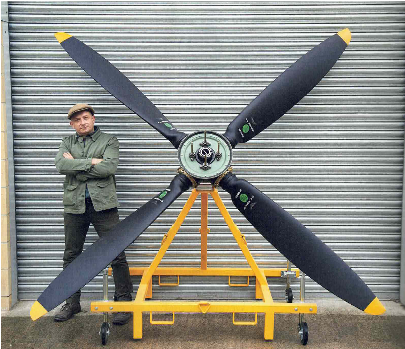
Hercules founder Rupert Wasey with one of his company's new, all-British Spitfire propellers
