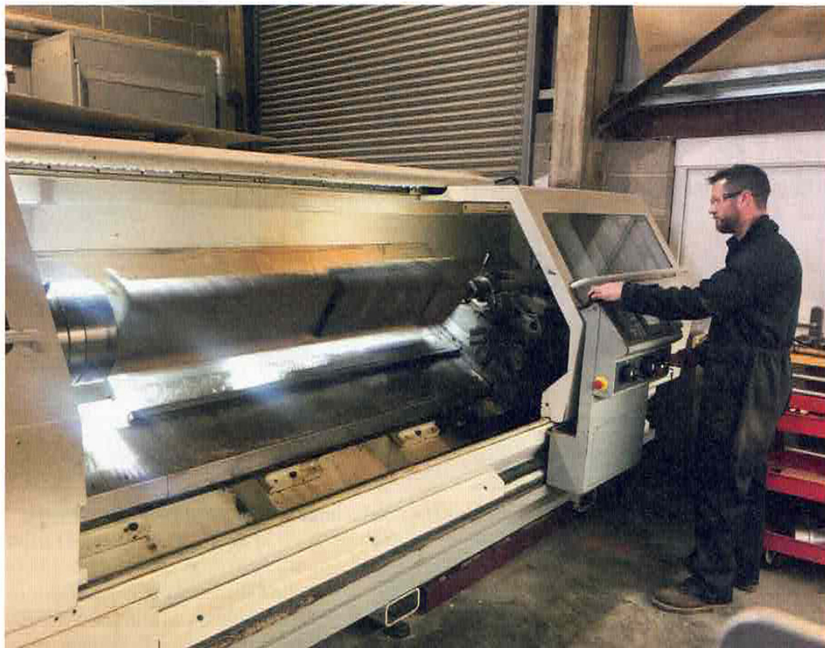
Using a huge lathe bought especially to do the job, a thread is cut in the blade root
