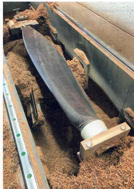
Blade shaped in Hercules's CNC milling machine
