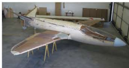
The almost completed airframe of the Le Reve Bleu LLC Bugatti 100P aircraft (Photo: Le Reve Bleu LLC)
