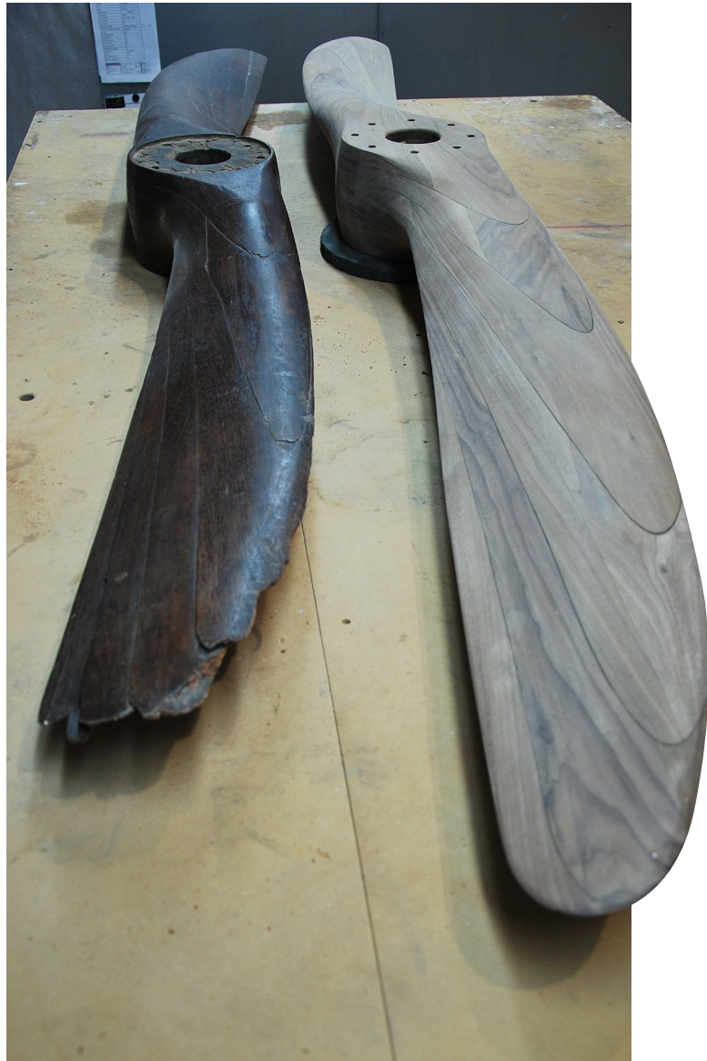
(Above) It is possible to recreate a prop from a damaged original. This is for a WW1 SE5a.
