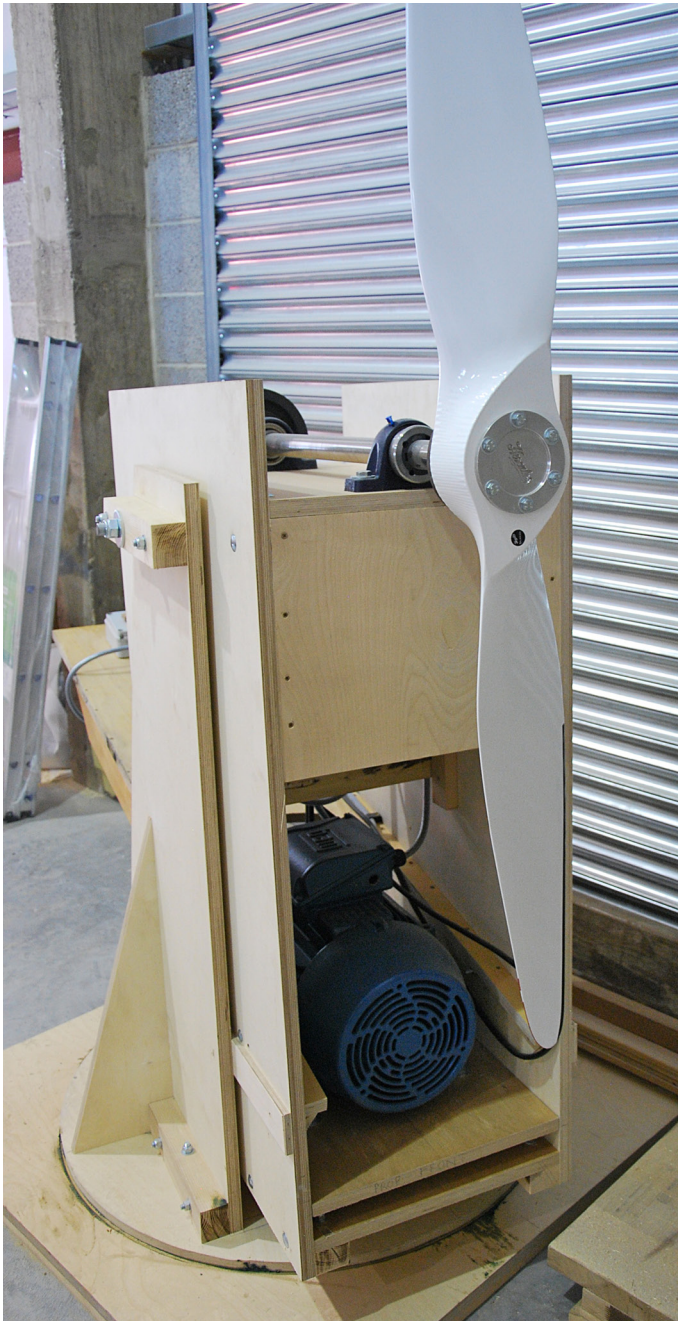
(Above) It is possible to recreate a prop from a damaged original. This is for a WW1 SE5a.
