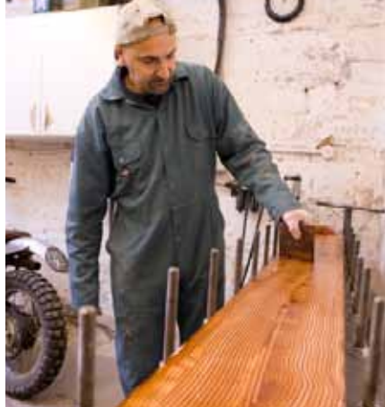
Left: George applying the Aerodux glue before the beech sections are clamped together. Below left: Rupert demonstrating the innovative design programme. Below: as well as building new propellers, Hercules can replicate existing designs, something that is particularly popular with owners looking to maintain the historic accuracy of their aircraft
